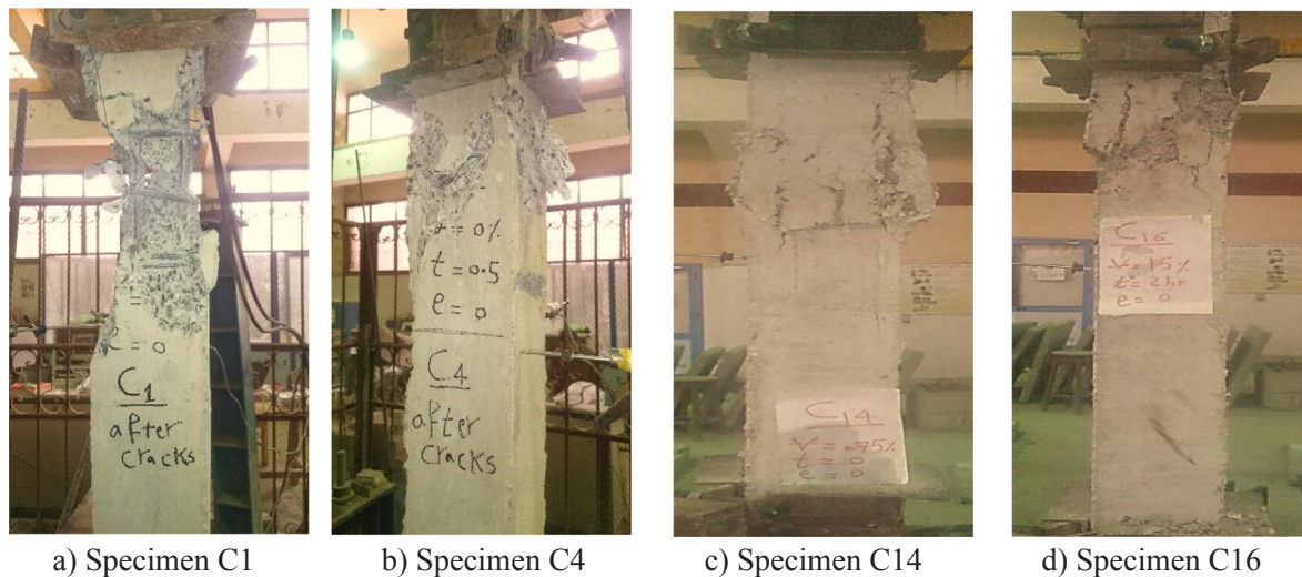
Fig. 4. Crack pattern and failure of columns tested under concentric loads.
